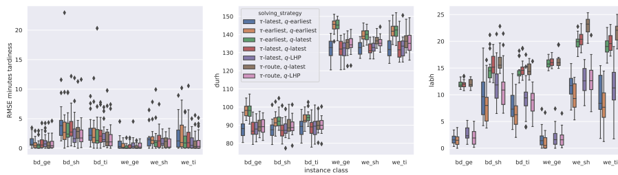
Fig. 5 Comparison of the root mean square error of the tardiness in minutes, the travel time duration, and the excess labor time of different solution strategies (without offline solution) on six different instances classes with 20 instances each. We observe that the more sophisticated strategies based on LHP and the route performance decreases the tardiness at the cost of carefully introducing additional travel time (regarding which \tau -latest is best) and labor time (where q -earliest is best).
